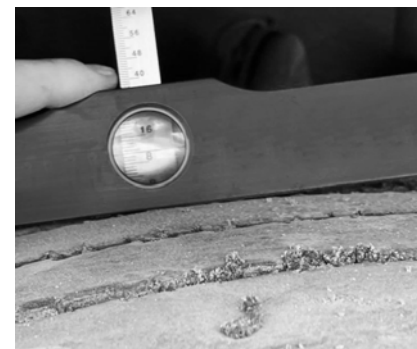
Tyre tread measured at 139,320kms
