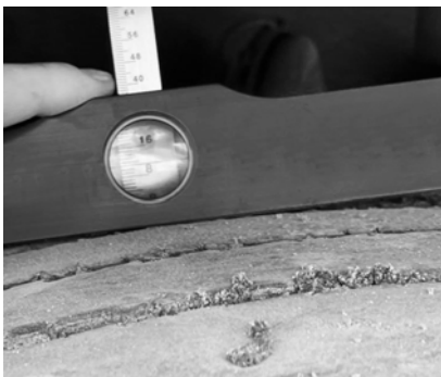
Tyre tread measured at 139,320kms
